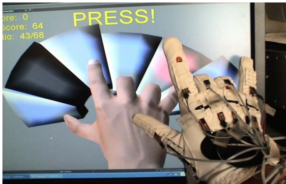
Fig. 2. Picture of the virtual keypad and hand, with the PneuGlove in the foreground.
